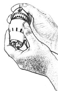
Do not tamper with the position of the bulb for any reason, in order to avoid loss of calibration of the thermostatic head.
